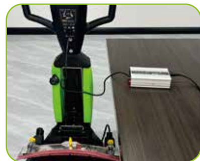
12. Charging the machine direct attachment
