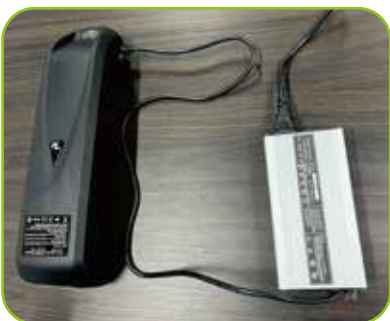
11. Charging batteries (Do not charging on concrete floors)
